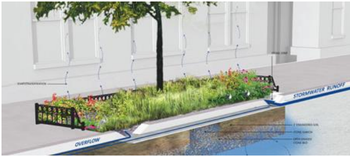
Example of a roadside bioswale
